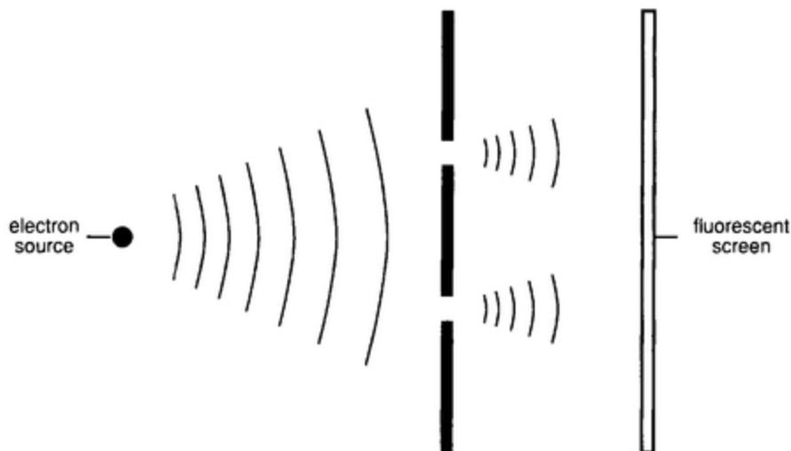
*Figure 14.* The double-slit experiment for electrons.
