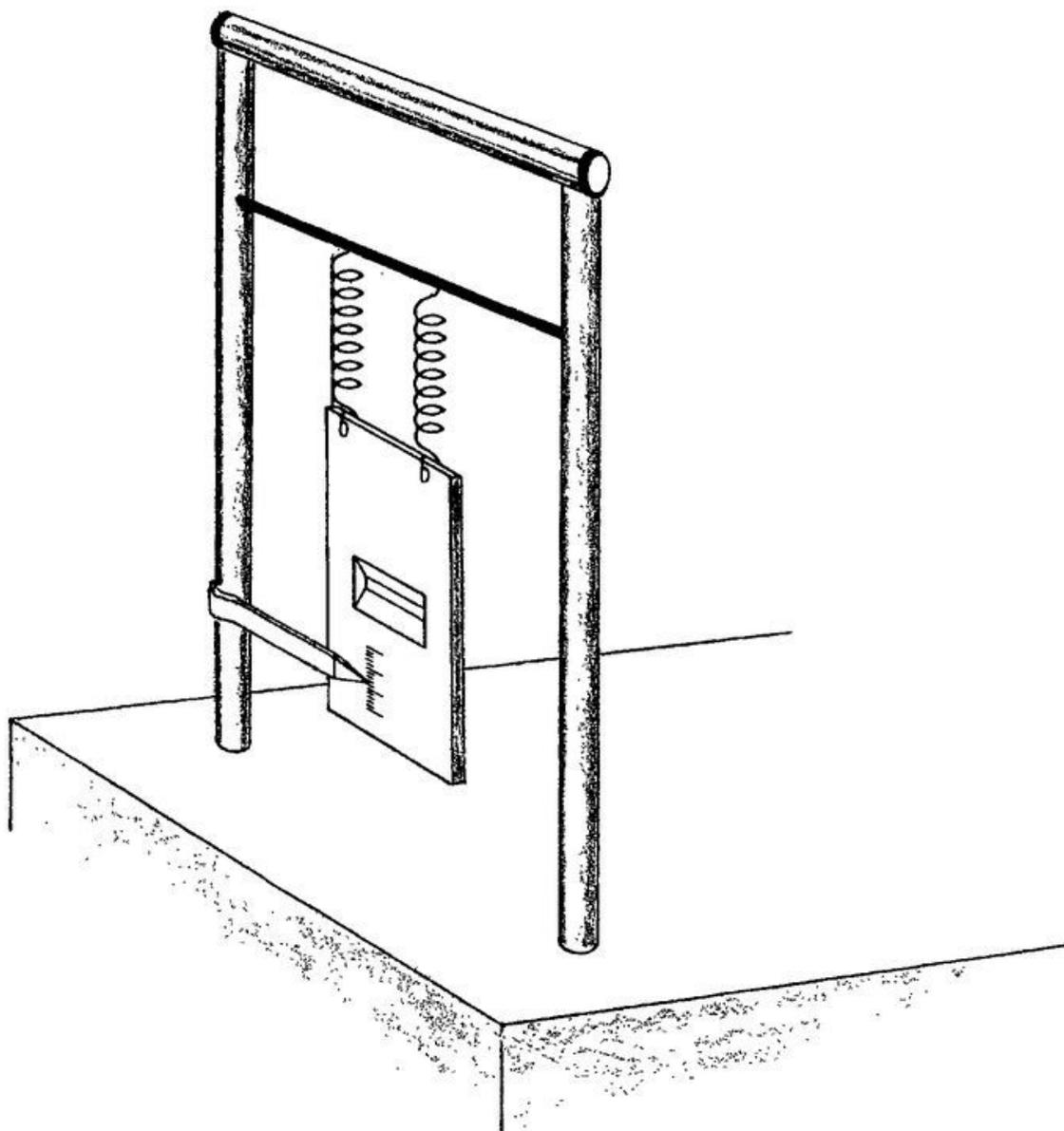
*Figure 24.* Einstein's spring-mounted initial slit for the double-slit experiment. If electrons go through a slit mounted on springs, as shown, before going through the double-slitted screen (not shown), is it possible to tell which slit an electron goes through without destroying the interference pattern?
