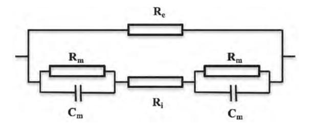
A schematic diagram of the electrical circuit formed as the biology of a single human cell. In the drawing,  $R_{\rm m}$  and  $C_{\rm m}$  indicate impedance for the cellular membrane. C indicates a capacitor, R indicates a resistor, and the sub m indicates that those properties are describing the membrane of the cell. Adapted from the Bangladesh Journal of Medical Physics.
